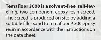
Temafloor 3000 is used for new and old concrete floors that need to resist strong chemical stress and high levels of mechanical abrasion. The product is ideal for laboratories, clean rooms and floors in the food and pharmaceutical industries, and for floors subject to heavy wear in production facilities. The components of the Temafloor 3000 system are base, hardener and filler sand.
