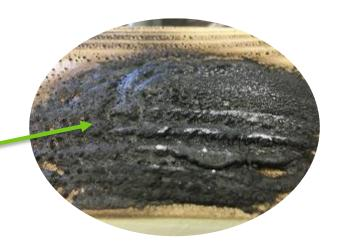
Intumescent coating creates a spongeous, porous layer. This layer has very good heat insulation properties.
